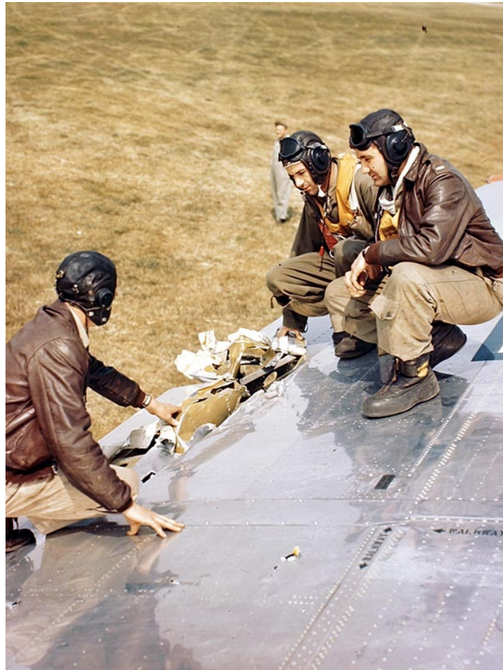
Back at base a crew marvels at the hole in their wing. According to Hal Landaker, who was the radio operator on this aircraft (the B-17 Sugar-Jo , assigned to the 550 th Bomb Squadron, 385th Bomb Group), the damage was received on a mission to Hannover Germany on 6 December 1944 when a direct hit from an 88mm.anti-aircraft shell that went completely through the wing, severing one of the main spars and exploded above the aircraft. Image 8221a, NARA 2016 Folder, EAAWP.
