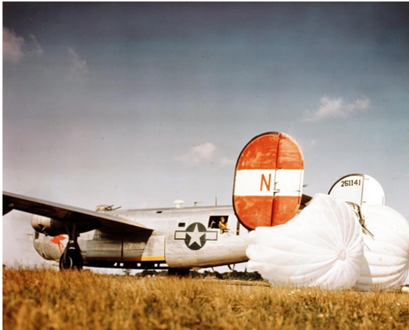
When the hydraulic system was shot out during a mission, the pilot landed his Consolidated B-24 at his base at Attlebridge in County Norfolk with two parachutes attached to the waist window to compensate for brakes. Image 8359a, NARA 2016 Folder, EAAWP.
